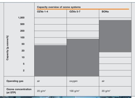
Ozone is the strongest disinfectant and oxidant permitted for water treatment. With an environmentally-friendly production process using air or oxygen, it decomposes to oxygen after use. The concentration can be measured online at any time. The optimal solution for swimming pool water, potable water, for the beverages industry and other industrial applications. ProMinent offers systems together with accessories in almost all sizes.
